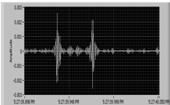
Fig. 13. Detection and localization of swell in pure sine wave using WPT
