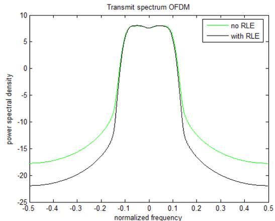
Fig. 3. Power spectral density
