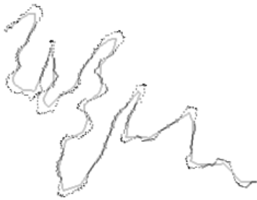
Fig. 3. Preservation of line characteristics for the improvement algorithm. The result is very close to original line while also nicely smoothed. ( SS=5 , SI=10 , SP=15 )
