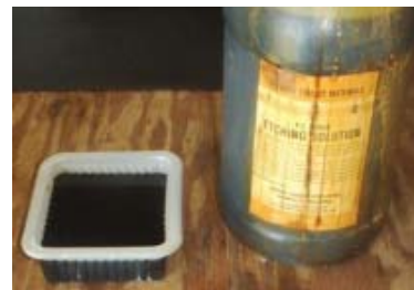
Fig. 9 Etching process using the ferrite chloride
