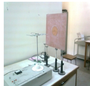
Fig.16 Setup for Testing an Antenna
